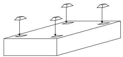
Figure 3-1. Attaching self-adhesive feet for desktop installation
